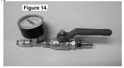
If a leak is found to be present, spray a soap and water mixture onto the bulkhead air fitting.
