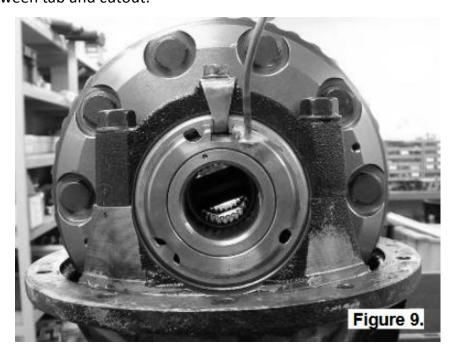
Install the spring clip by first hooking both ends of the clip into the small aligned cutouts of the seal housing and the adjuster nut, and then snapping the clip into the groove of the seal housing using a screw driver. (Fig.10.)
