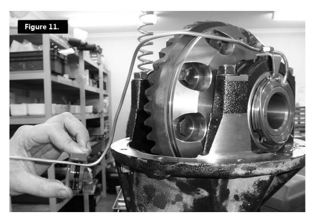
NOTE: Use an automotive brake line tubing cutter to cut the seal housing tube, never a hacksaw as this will leave metal filings in the air system.
