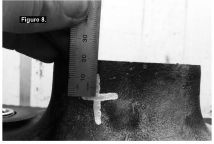
NOTE: To best determine the correct vertical position of the drilled hole, measure down from the machined face (shown at the top of the picture in Figure 8.) a distance of 19mm [3/4"] and mark the horizontal line which the hole is centered on. Then refer to Figure 9. for the correct position on that line to start drilling.
