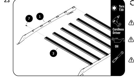
Assemble the Footrails (Item1) to the six rear slats (Item 3) (Leave the first slat unassembled for now) using M6 x 25 Thread Forming Screws (Item 7).
