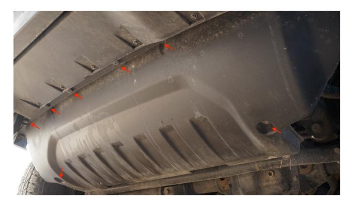
Clips are a two-piece design. Using a pry bar or trim clips tool lift the inner piece about 1cm and then remove the whole clip. Some significant force is required here as this place gets quite dirty.
