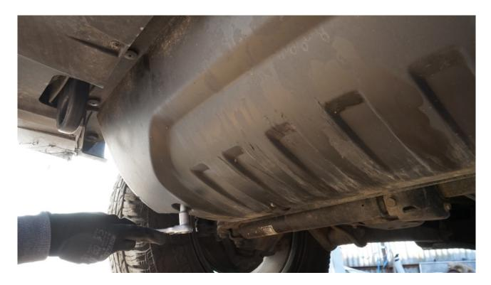
Using a 7 mm socket wrench loosen and remove 7 fasteners holding inner plastic covers on both sides of the bumper.
