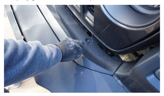
The same trim piece is also held by white clips from inside the bumper. Release them by pinching them and pushing up. Use long needle nose pliers for best access.
